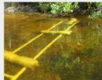
Figure 3. RFID PIT tag array deployed in the river.
