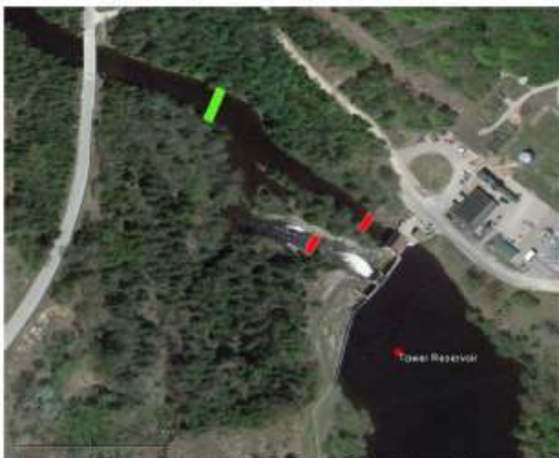
Figure 2: Aerial map showing the location of PIT-tag interrogation systems near Tower Dam. Green rectangles represent PIT-tag interrogations systems that were fully operational for this 2014 pilot study, while the red rectangles represent PIT-tag interrogation systems that will be fully operational in 2015.
