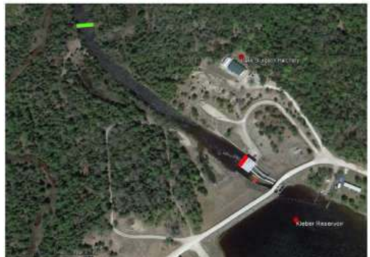
Figure 3: Aerial map showing the location of PIT-tag interrogation systems near Kleber Dam. Green rectangles represent PIT-tag interrogations systems that were fully operational for this 2014 pilot study, while the red rectangles represent PIT-tag interrogation systems that will be fully operational in 2015.
